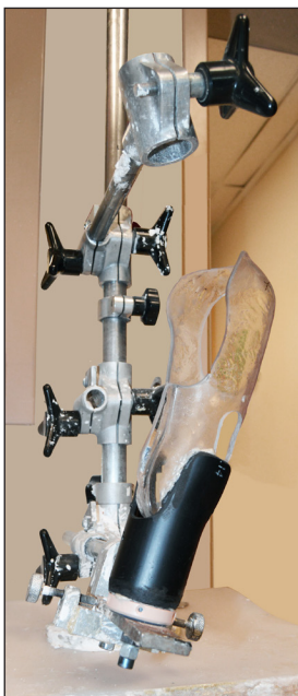
Figure 4 - Vertical Transfer Fixture with temporary alignment fixture fabricated from PVC.
